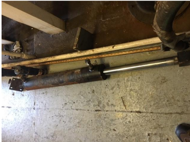
Left, the port flanking rudder steering hydraulic ram that was removed after the incident. Right, the port flanking rudder steering system with the original steering ram in place.
