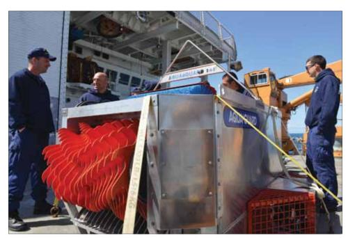
Crew members aboard Coast Guard Cutter *Healy* prepare an ice-capable oil skimmer for testing in the Arctic in July 2017. The Coast Guard Research and Development Center often deploys existing oil spill response technologies to better understand limitations and capabilities, especially in the Arctic. U.S. Coast Guard photo by Senior Chief Petty Officer Rachel Polish.
