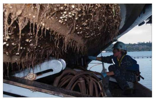
A sailor scrapes barnacles from the bottom of a rigid-hull inflatable boat aboard the aircraft carrier USS *John C. Stennis*. U.S. Navy photo by Seaman Apprentice Christopher Frost.
