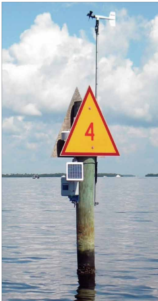
Meteorological Instruments on Coast Guard Aid to Navigation: Aerovane (wind speed and direction), air temperature, data logger with internal pressure sensor, as well as a solar panel and box inclosing battery, cell phone modem and CPU. Photo courtesy of WeatherFlow
